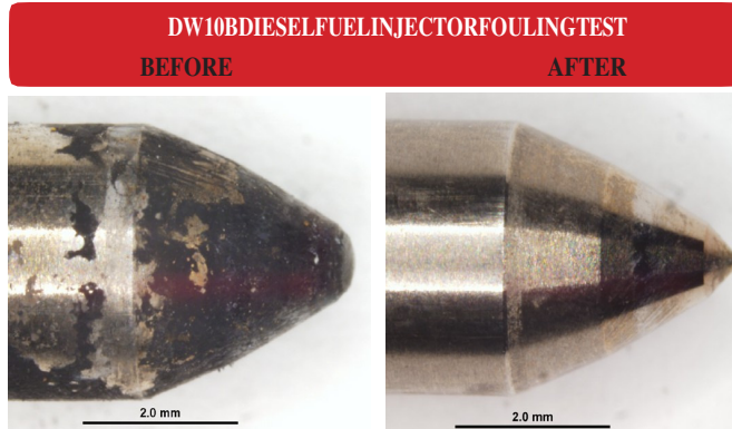
High Pressure Common Rail injectors before and after clean-up with fuel treated with Diesel ECP + Cetane Boost.
